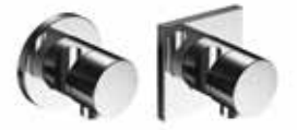
59548 3-way diverter valve with wall outlet for shower hose and hand shower bracket DN 15 Set complete with: handle, casing, rosette (round or square) and diverter valve, intrinsicly safe against backflow, suitable for rough part no. 59548/000170
